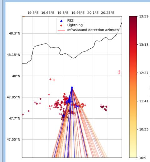
The figure on the left shows an example of a storm close to PSZI on 30.08.2019. Lightnings are marked with crosses and infrasound detection azimuths are represented with lines. Both are color-coded by time. Those infrasound detections that are associated with EM detections are colored with blue. Note that one infrasound detection might belong to multiple EM detections due to uncertainty.
