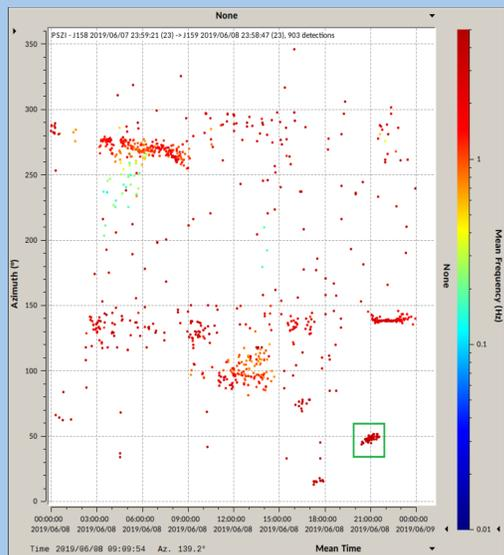
The figure on the left shows PSZI infrasound detections visualized by DTK-DIVA (part of the CTBTO NDC-in-a-box software package) on 06.08.2019. The points are color-coded by frequency. The green box in the bottom right marks the detections that are connected to a storm.
