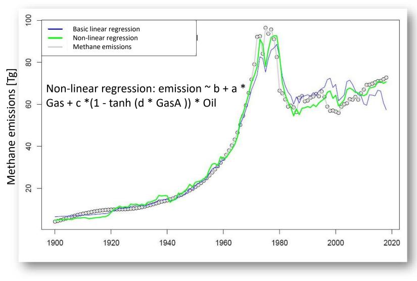
Basic linear regression (~ b + a \* Gas + c \* Oil, blue line) failed over the whole time scale. Additionally bad is the negative *a* (b = 5.7, a = -0.053, c = 0.041)
