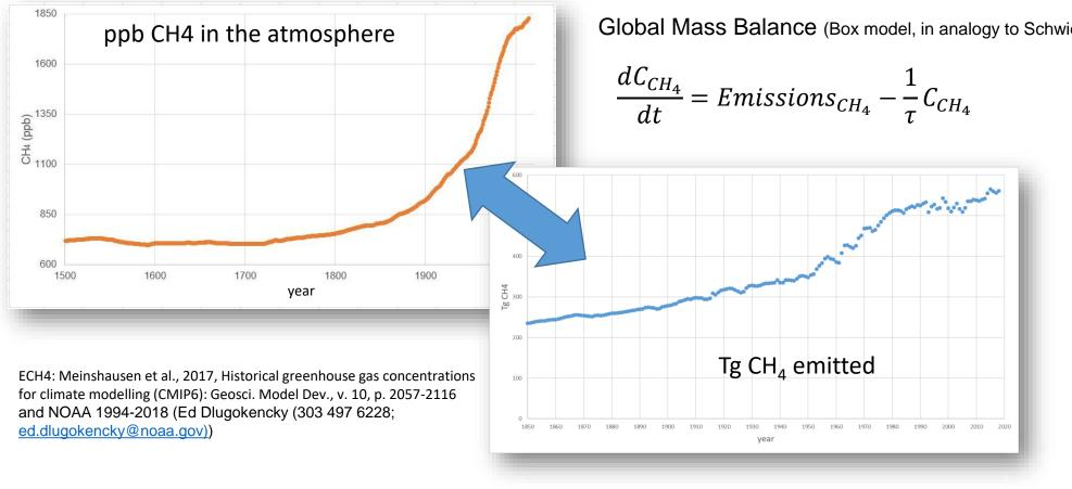
Global Mass Balance (Box model, in analogy to Schwietzke et al., 2014):
