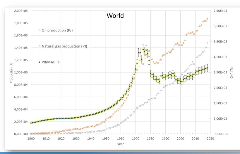
Globally oil production globally initiated earlier with respect to than natural gas production (~1950ies). We test the correlation of O&G production with methane inventories using regression models for global and regional data.
