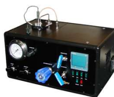
Fig. 10 - UCA (ultrasonic cement analyzer)
