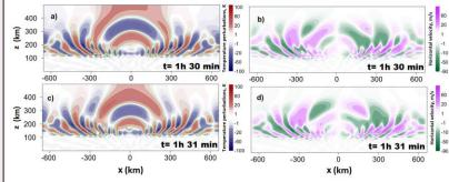
These simulations show that the amplitude of the wave temperature disturbances in the upper atmosphere is approximately 100 K, and the amplitude of the horizontal velocity is 60 m/s. In addition, in the upper atmosphere, a heated zone forms above the source approximately two hours after its activation. This heated zone is most likely formed by very long infrasonic waves propagating very slowly upward from the source due to their properties.
