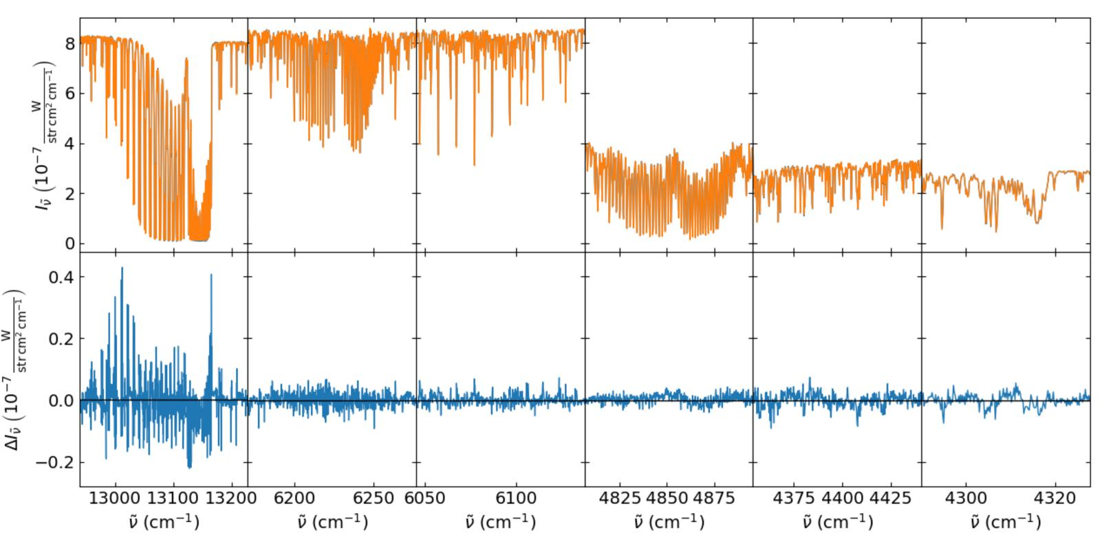
Averaged spectrum of 100 measurements  $I_{\tilde{\nu}}$  (orange) and spectral residuum  $\Delta I_{\tilde{\nu}}$  (measured – modeled, blue) with, from left to right,  $O_2$  A-band, weak  $CO_2$  band,  $CH_4$  band, strong  $CO_2$  band, and new GOSAT-2 retrieval windows for N<sub>2</sub>O (4354–4441 cm<sup>-1</sup>) and CO (4290–4328 cm<sup>-1</sup>). Different versions of the instrument line shape can not reduce the large spectral residuum.
