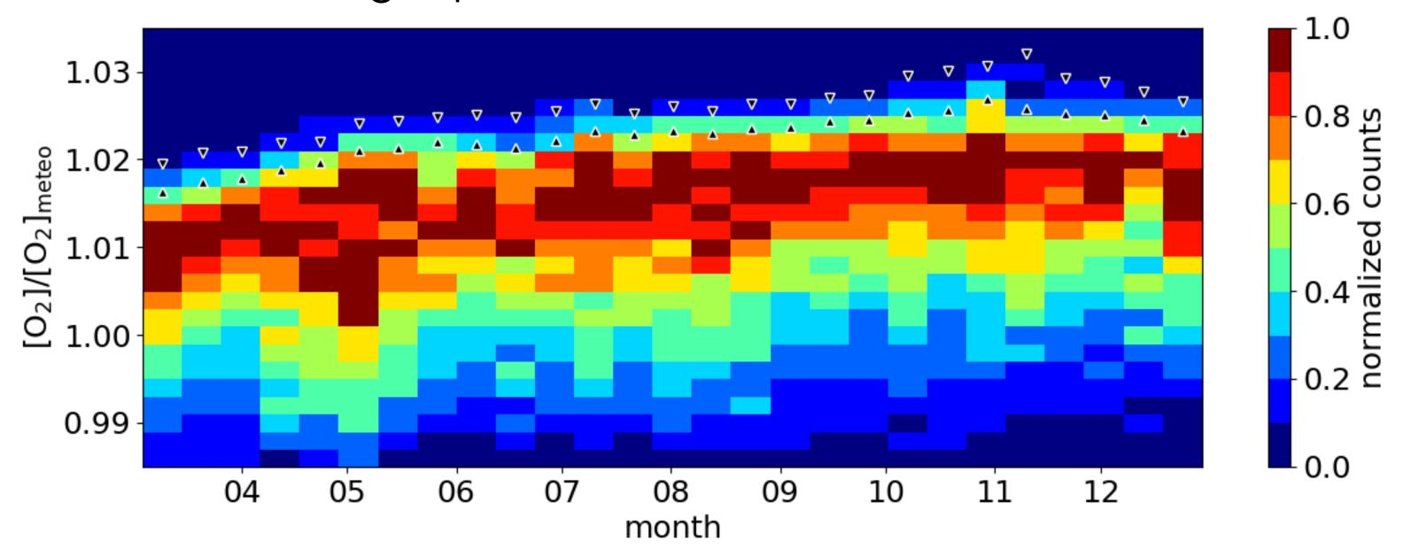
Retrieved oxygen column in ocean-glint geometry over 10 months in  $\sim$  10 days-bins. Each bin shows a normalized, color-coded histogram. **Temporal variability** is obvious both in the peak (dark red) and in the upper-edge ensemble of clean soundings (1) (black triangles).
