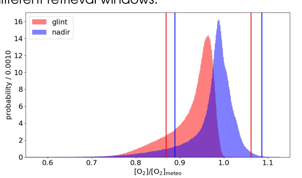
Exemplary histogram of the  $O_2$ -ratio with the criteria of the coarse cloud filter shown by vertical lines.
