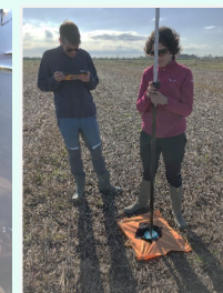
Measurement of GCPs and CPs through a GNSS
