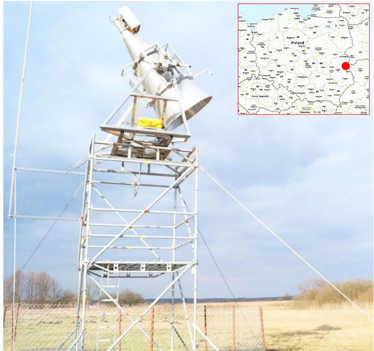
In 2016-2019 we conducted 16 field campaigns. We measured surface soil moisture in situ using TDR, and interpolate it to semicontinuous grid using geostatistics. Then, the driest and the wettest points (in space and time) were chosen and assigned to, maximum and minimum thermal inertia, respectively. Basing on that, the model retrieving soil moisture was built, and the other measurements served as evaluation assembly.
