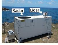
35 GHz Ka-Band cloud Doppler radar is used to measure the vertical velocity of the cloud droplets. It has a sensitivity of -52 dBZ at 5 km and a temporal resolution of 10 s. The Doppler resolution is < 0.02 m s<sup>-1</sup> between  $\pm 10$  m s<sup>-1</sup>.
