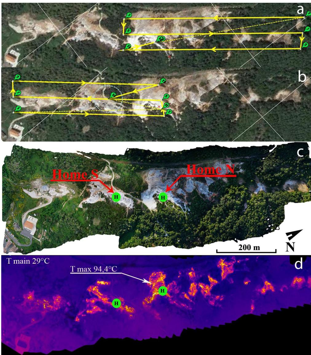
UAV flight of 18 June 2019 on the *Parco delle Biancane*: a) flight plan for the northern sector; b) flight plane for the southern sector c) visible mapping; d) thermal mapping. The “Home” (H) indicates the take-off point of the UAV which has a ground elevation of 621m and 610m in the northern and southern sector respectively.
