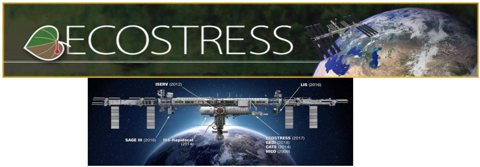
**ECOSTRESS(from 2018):** Five channels in the thermal infrared region with spatial resolution of about 38x68m at nadir and revisit time of 5days. From May 2019 8.29  $\mu\text{m}$  and 9.20  $\mu\text{m}$  are not available
