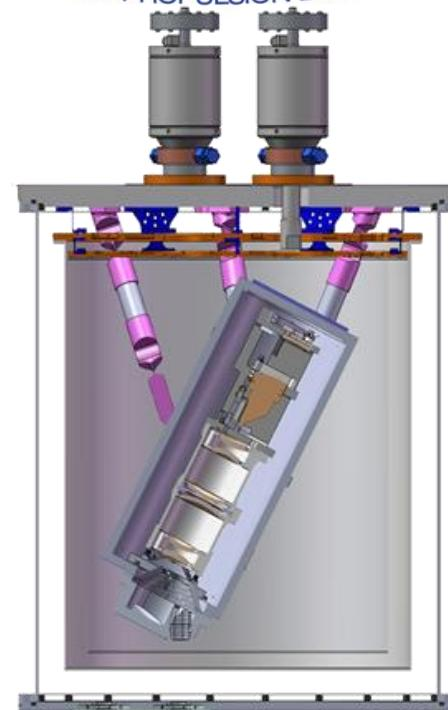
HyTES is a compact image spectrometer acquiring data in 256 spectral bands between 7.5 and 12 micrometers.
