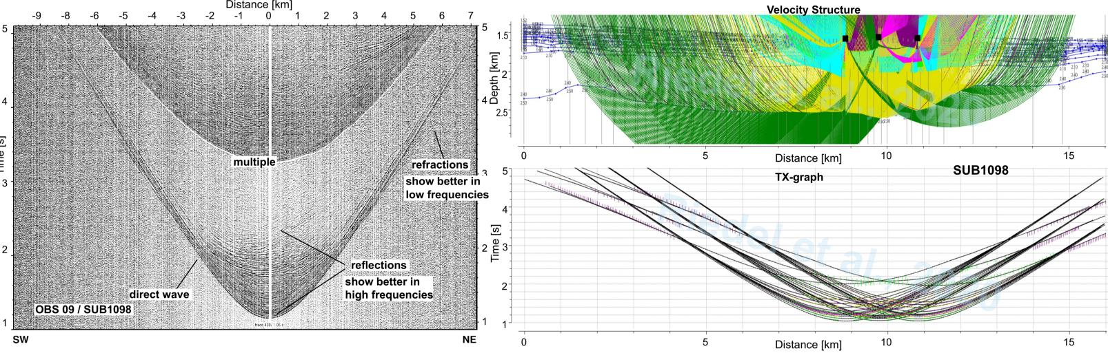
Velocity structure: Note higher ray density, and therefore model resolution in the center beneath OBS stations (cubes). TX-graph: Vertical colored lines are picked reflections/refractions; black lines are calculated traveltime curves.
