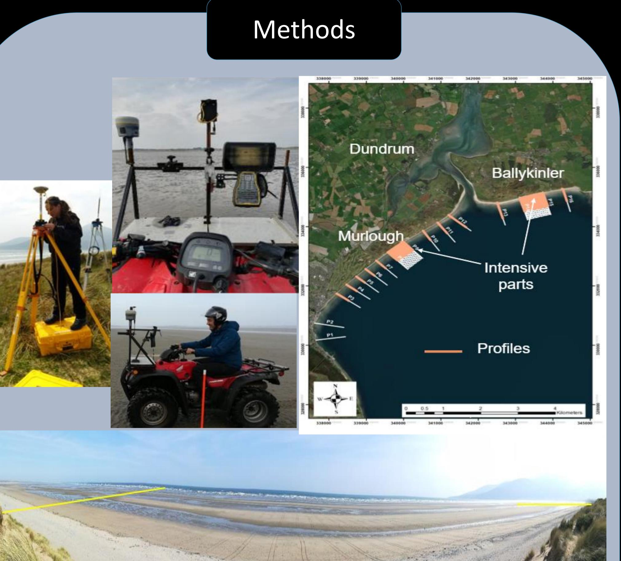
Monthly intertidal topographic surveys now underway > 2 quadbikes equipped with RTK-GPS > 10 profiles at Murlough beach > 4 profiles at Ballykinler beach > 2 intensive part (10 m spaced lines) on both sites
