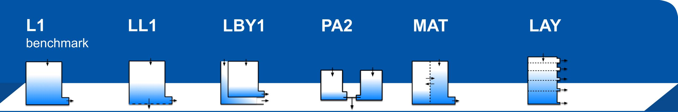
Simple linear storage (L1) as benchmark model with recharge as input and baseflow as output. Storage coefficient k controls drainage.
