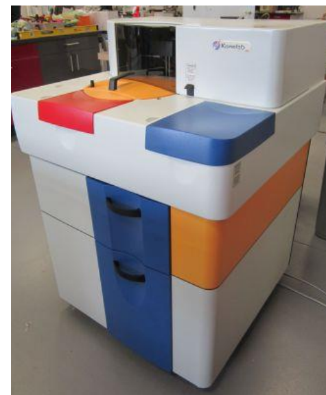
Cl concentrations double-checked using Thermo F. Scientific Konelab analyzer
