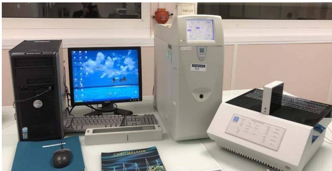
Analysis of Cl and Br using IC Dionix ICS-1500 with AS40 automated sampler
