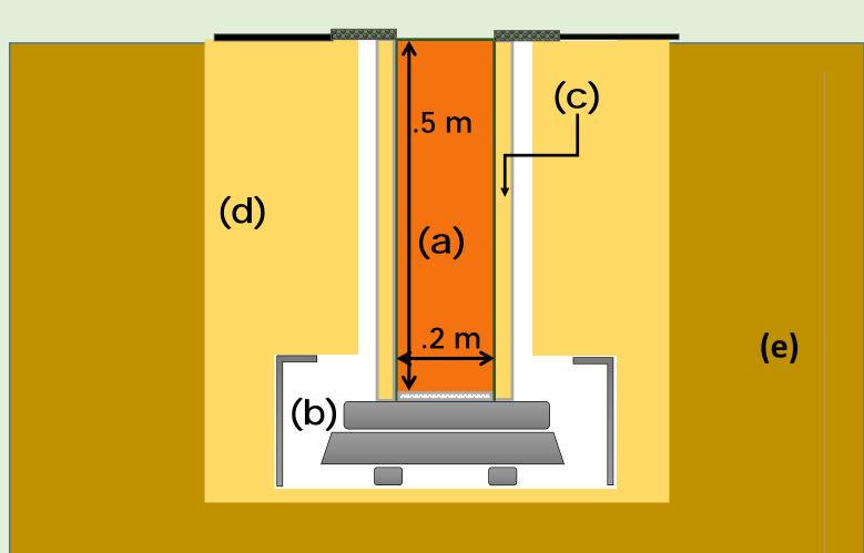
SCHEMATIC VIEW OF MICRO LYSIMETER (M-L)
