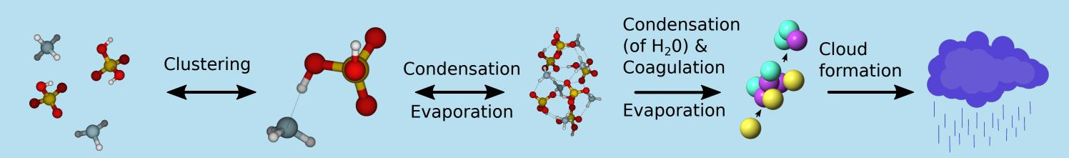
Computational studies can reveal the role of specific atmospheric compounds (here: sulfuric acid and ammonia) in the growth path from single gas molecules to bigger molecular clusters and shed light onto their role in cloud formation.
