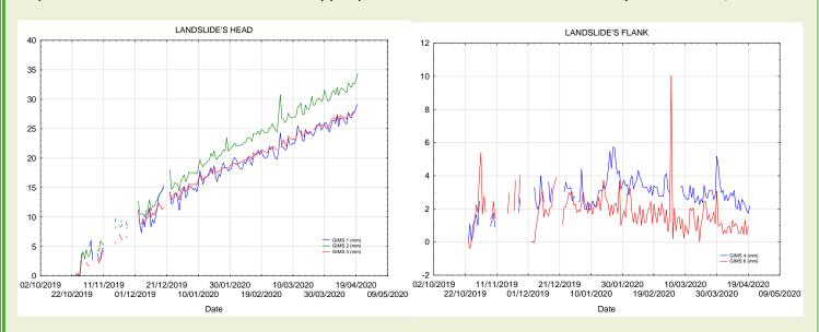
The flank of the landslide that is being monitored by GIMS units 4 and 6 exhibits negligible displacement. This area currently does not show active displacements.
