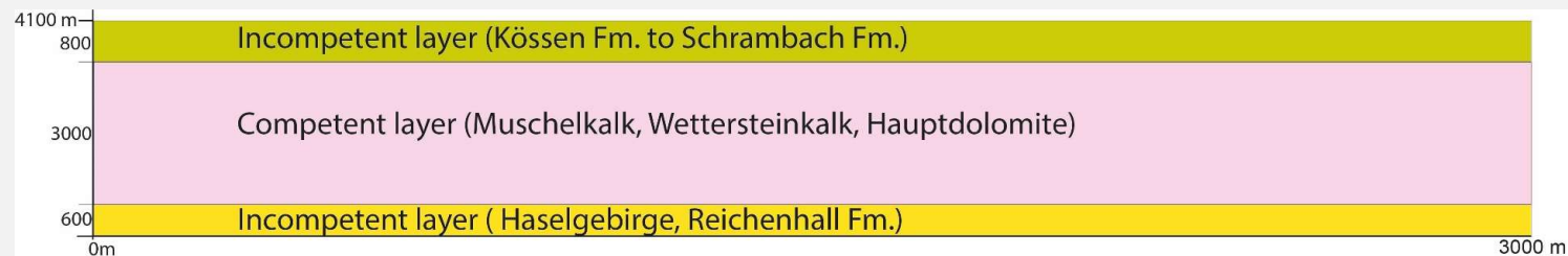
Fig. 2: Simple 3-layer model for the numeric simulation based on the stratigraphic knowledge of the NCA.
