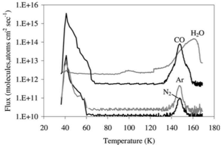
Fig. 1. A plot of the fluxes of evolved CO, N<sub>2</sub>, Ar and water during warming up of 0.1 μm ice layer. The gas-laden ice was deposited at 27 K from a H<sub>2</sub>O:CO:N<sub>2</sub>:Ar = 100:100:14:1, at a rate of 5 × 10<sup>-4</sup> μm min<sup>-1</sup>. At 35–65 K the gas frozen on the ice sublimates. The internally trapped gases are released at 135–160 K during the transformation of the amorphous ice into a high viscosity “liquid” with cubic domains.
