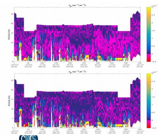
Before the correction of Kray and Kmie : due to an underestimation of these coefficients, inverted backscatter coefficients tend to be negative and particle-free regions of the atmosphere.
