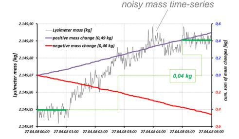
A filter is required to separate background noise from real lysimeter mass changes. Without applying a filter, the pos. mass changes in the example above would result +0.49 kg and the neg. mass change would result -0.46 kg, which is equal to 0.49mm P and 0.46mm ET (no leachate recorded in this example). In fact, there was no ET (→ night) and also no precipitation was recorded by nearby standard gauges. The +0.04kg real mass increase between 0am and 6am resulted from dew.
