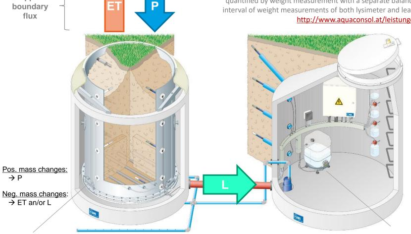
Load cells resolution of weighing system  $10g \rightarrow 0,01$ mm
