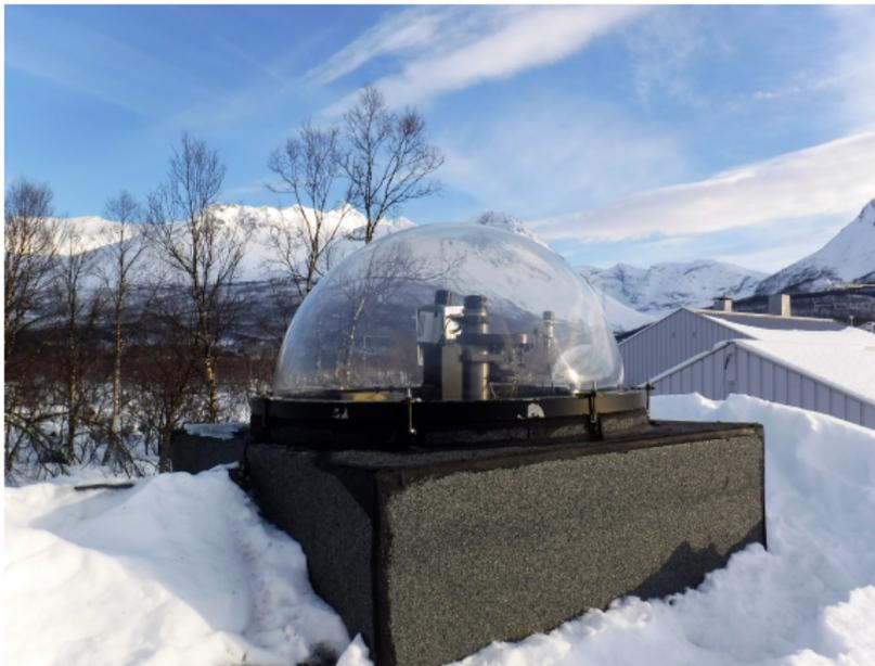
**Figure:** Running in parallel a few 100 metres from the radar control room are an iXon-888 EMCCD camera mounted with a 427.8 nm filter, and pointing into the magnetic zenith ( $az=180^\circ$ ,  $el=77^\circ$ ) with a  $30^\circ$  field of view (FOV). An ALTA-U47 back-illuminated CCD camera was mounted with a 844.6 nm filter, and pointed into the local zenith with a  $50^\circ$  FOV
