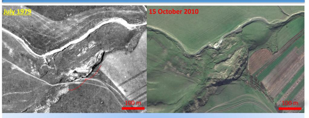
After 2005, the scarp slumping continued, but in the same time the increased Miletin river channel sinuosity started to erode the basal part of the landslide. The evolving channel sinuosity and erosion has created stability of the landslide body, the previous scarp slump deposits being mobilised. The scarp has shown new signs of slumping.
