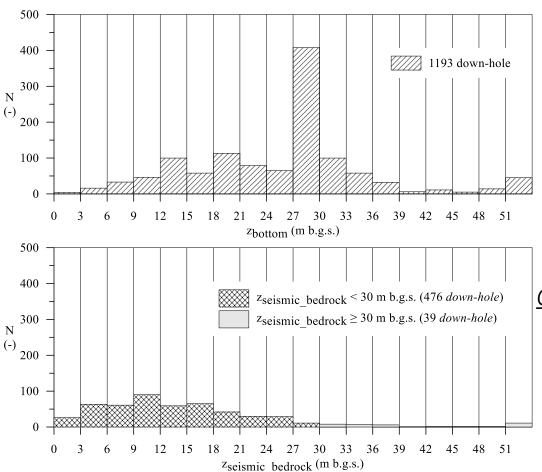
Geophysical surveys are generally extended down to 30 m b.g.s.
