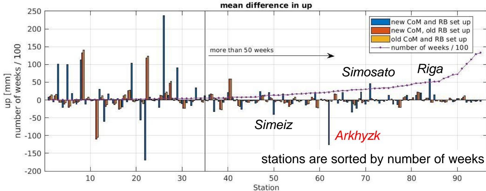
Partly large changes of individual station positions due to global range bias estimation (all components are affected, but station height most).
