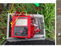
2) 2D-ERT Field installation UNI-T UT523A devise: 36 electrodes with 0,33 m spacing
