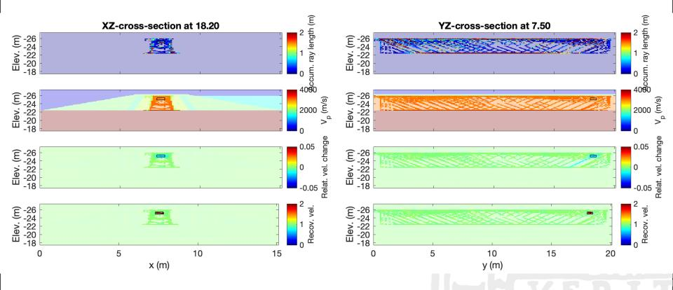
Cavity  $-\begin{cases} Size: 0.4 \times 0.4 \times 0.4 \text{ m} \\ V_p = 1000 \text{ m/s} \end{cases}$
