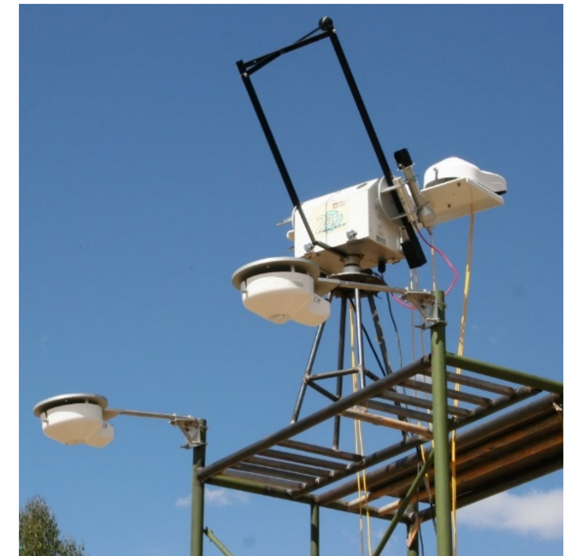
BSRN Station. (Baseline Solar Radiation Network). Measurement of Surface short wave and long wave solar radiation.
