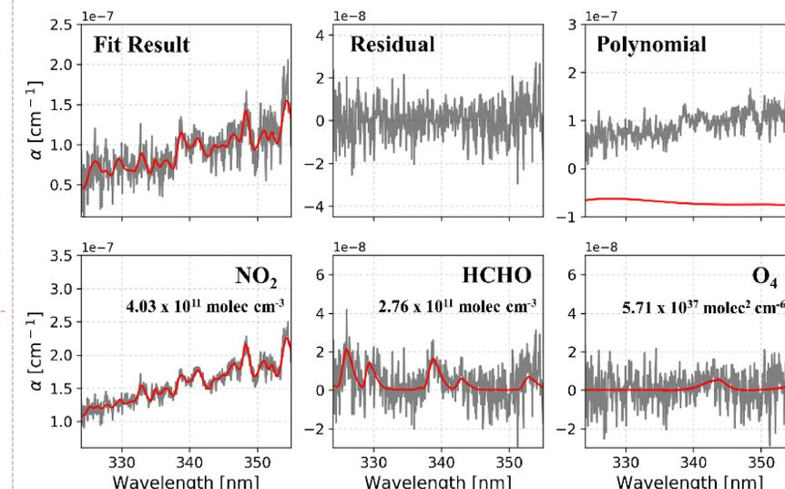
An example of spectral fitting for one spectrum (60 s average) measured during a field campaign on 15 August 2019 at 08:59. The red line represents the fitted spectrum, and the black line is the fitted result plus the residual. Corresponding NO<sub>2</sub> and HCHO concentrations is 16.4 ppbv and 11.2 ppbv, respectively.
