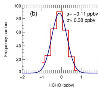
At an integration time of 30 s, the measurement precision ( $1\sigma$ ) for HCHO was 380 parts per trillion volume (pptv) and the corresponding uncertainty was 8.3%.
