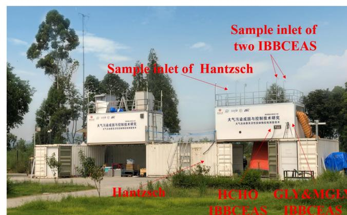
Measurement site in the Szechwan Basin and laboratory containers where the HCHO IBBCEAS, GLY&MGLY IBBCEAS, and Hantzsch instruments were deployed.
