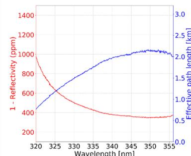
The reflectivity of the two cavity mirrors used herein was 0.99965 (1-reflectivity = 350 ppm loss) at 350 nm, which corresponded with an effective optical path length of 2.15 km within a 0.84 m cavity.
