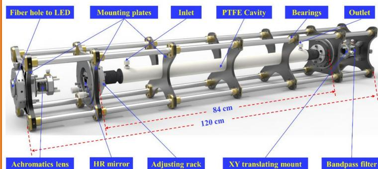
The entire cavity module adopts the cage structure design to enhance the system stability; this design is more convenient for replacing parts and adjusting the optical path, which can improve system reproducibility.
