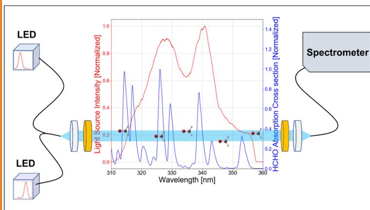
The optical layout of the IBBCEAS system consists of a light source module, an optical cavity module, and a spectrometer. Using two LEDs coupled by a Y-type fiber bundle as the light source is the core of the whole system.
