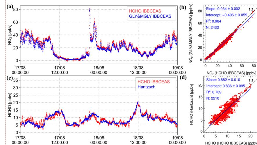
Partial data from the field campaign in the Szechwan Basin. (a) Time series of NO<sub>2</sub> concentrations measured by HCHO IBBCEAS and GLY&MGLY IBBCEAS. (b) Correlation plot for NO<sub>2</sub> measurements by two IBBCEAS. (c) Time series of HCHO concentrations measured by HCHO IBBCEAS and Hantzsch instrument. (d) Correlation plot for HCHO measurements.
