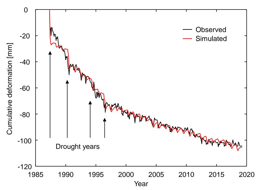
subsidence: Observed simulated Simulated and subsidence overall agrees with observed subsidence. Model successfully reproduced seasonal expansion and contraction. Significant subsidence is found in drought years, which reflects changes in groundwater demand.
