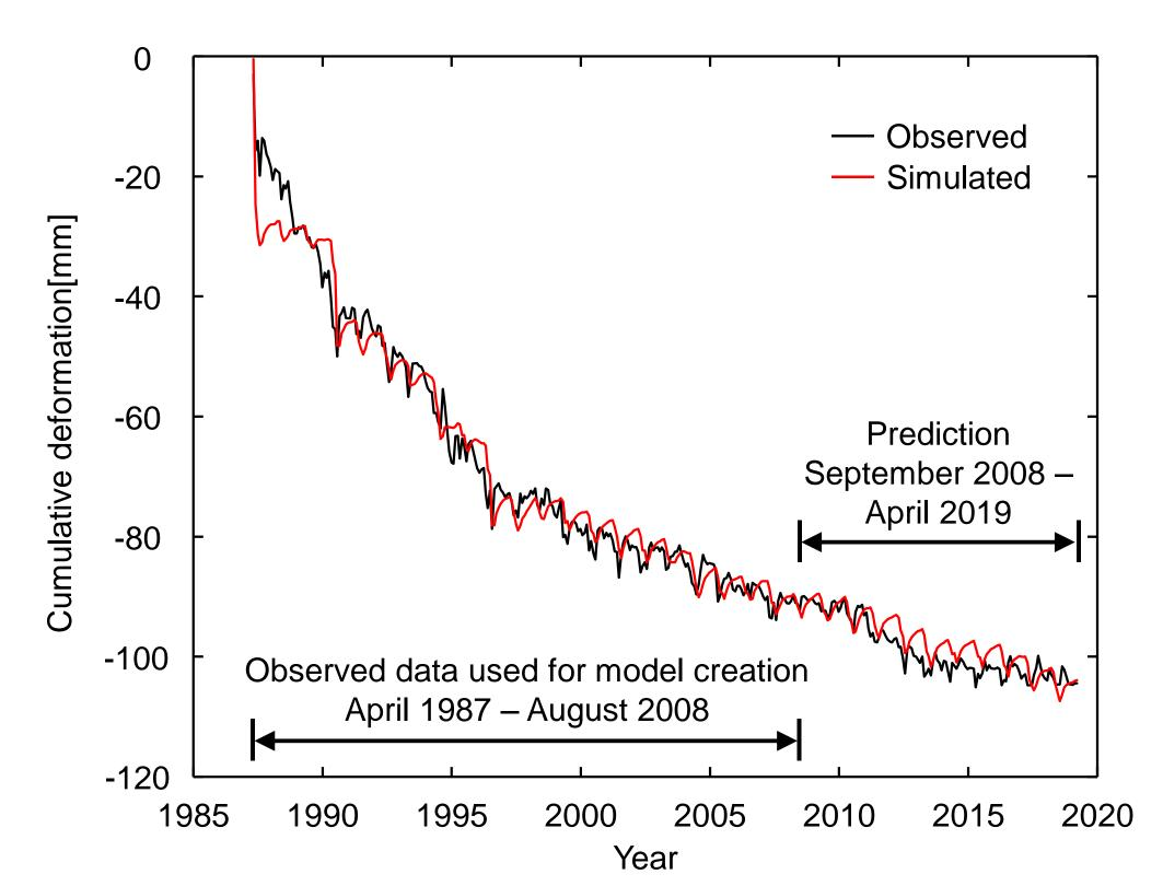
**Predictive errors**: To test model's predictive performance, another model was calibrated using the first two-thirds of observed data. Then, subsidence was predicted for the remaining one-third. The fit of the simulated and observed subsidence has not been good since 2011. One possible reason is the impact of land subsidence caused by the March 2011 earthquake.
