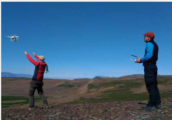
Figure 3. Left: Drone operators landing the UAV. Right: Operator measuring a GCP location with GPS
