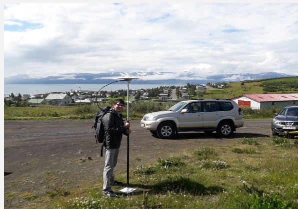
Figure 3. Left: Drone operators landing the UAV. Right: Operator measuring a GCP location with GPS
