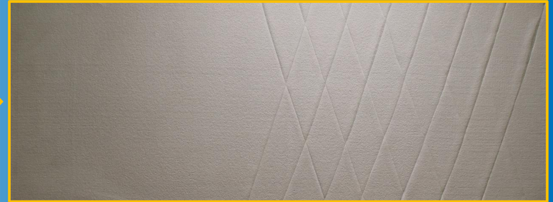
(b) Example of two discontinuity sets S1 and S2 cutting through the UC layer of a target model.
