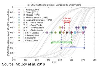
The temperature for which the liquid cloud fraction is equal to 50% (*T*<sub>50</sub>) from different Global Cloud Models variate by 35°C
