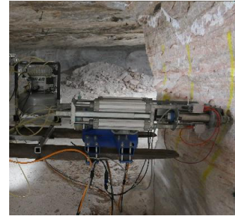
Left: Seismic vibration source systems around the pillar wall and right: within the observation wells.
