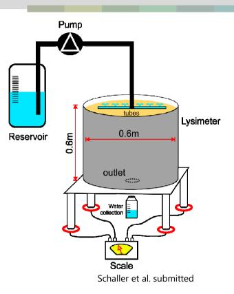
Lysimeter study using amorphous silica mixed with sand
