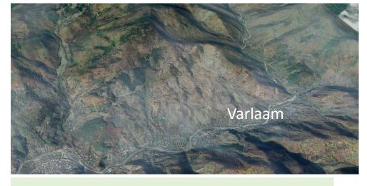
Varlaam is a massive slope landslide, reaching up to 2 km in length. It presents numerous shallow reactivation sectors across the body and is subject to river undercut along the toe, which is causing riparian reactivation. Surveys performed: seismic arrays + HV measurements.
