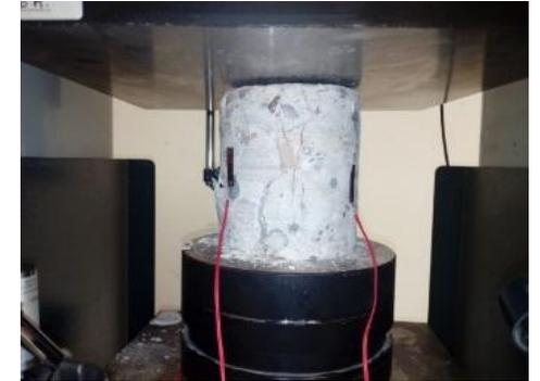
Test layout used in the uniaxial compression test of the concrete core-drillings. Image of the D3 sample at failure in compression
