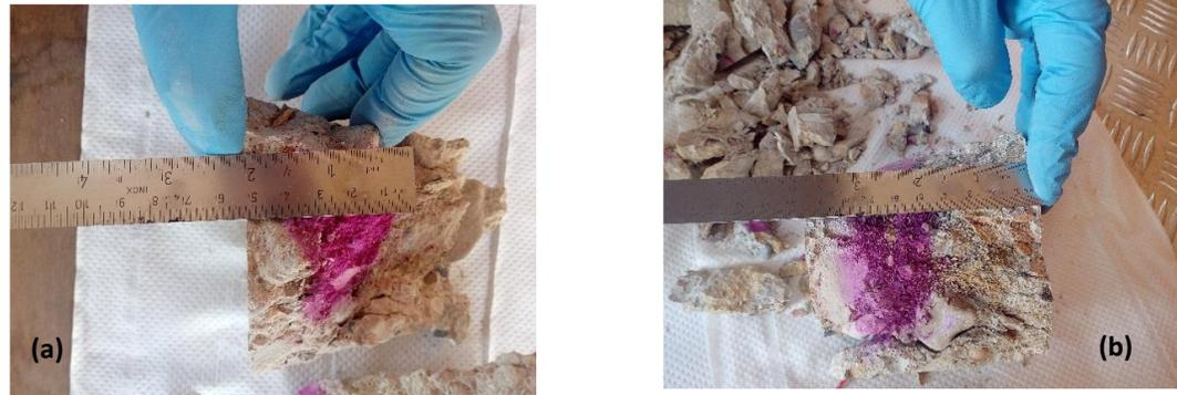
Results of the phenolphthalein indicator test for D3 (a) and D4 (b) concrete samples.
