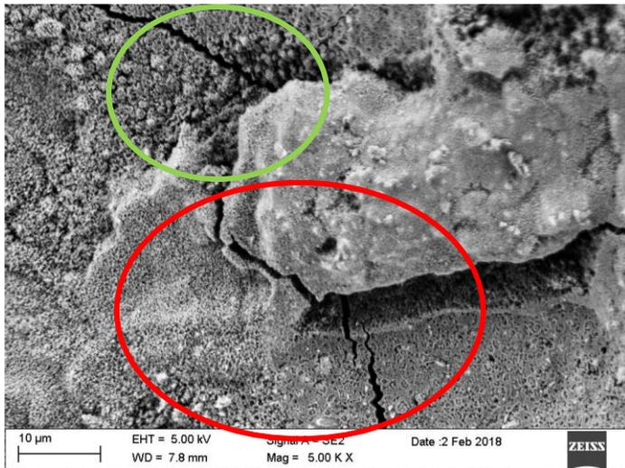
The SEM observation of the fracture surface showed a crack propagation both **transgranular and intergranular**, confirming the occurrence of a double mechanism exfoliation and stress corrosion.
