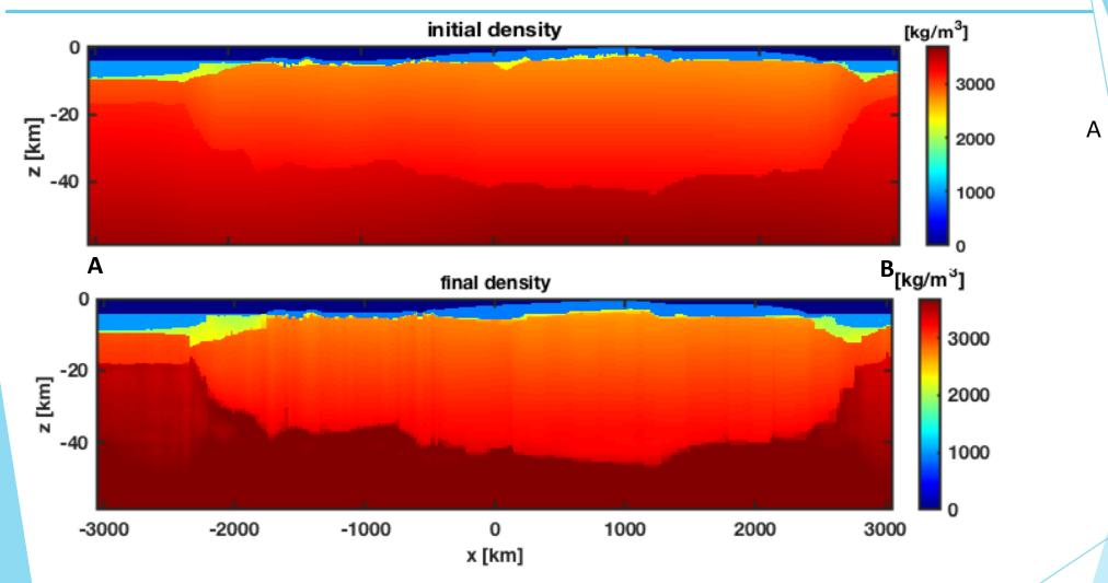
From this sections emerge that the algorithm increases the sediments and reduces the mantle density below the ocean ... BUT this is just a preliminary result!
