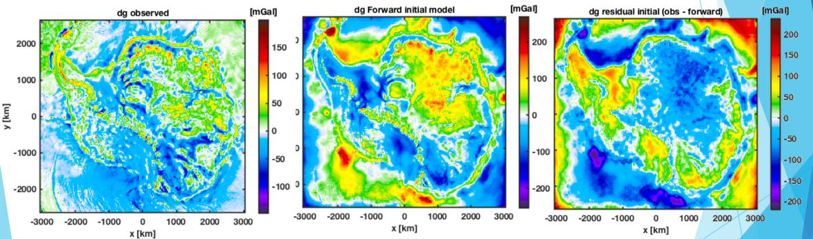
As shown in the third figure, the gravity signal generated from our initial model is quite different from the observed one with a std of about **64 mGal**
