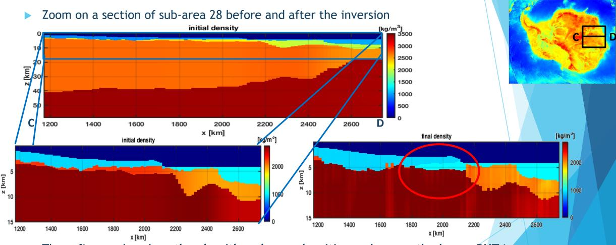
These figures show how the algorithm change densities and moves the layers BUT in this test, it generated a not physical situation (it segmented the sediment layer introducing water between the ice and the crust - in red circle)
