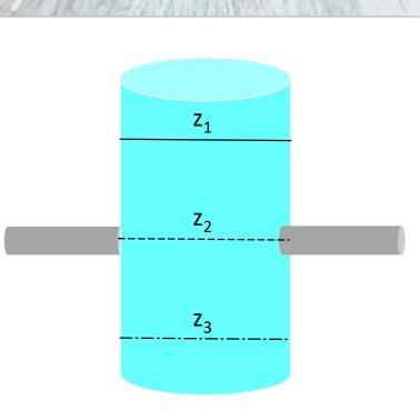
We obtained 3 measurements along a 10 cm long ice sample with an azimuthal resolution of 15°.
