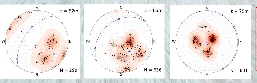
The colatitude angle of the pattern changes from 90° to 0° with increasing depth. The azimuth is aligned with the ice flow (ex. 2 m)
