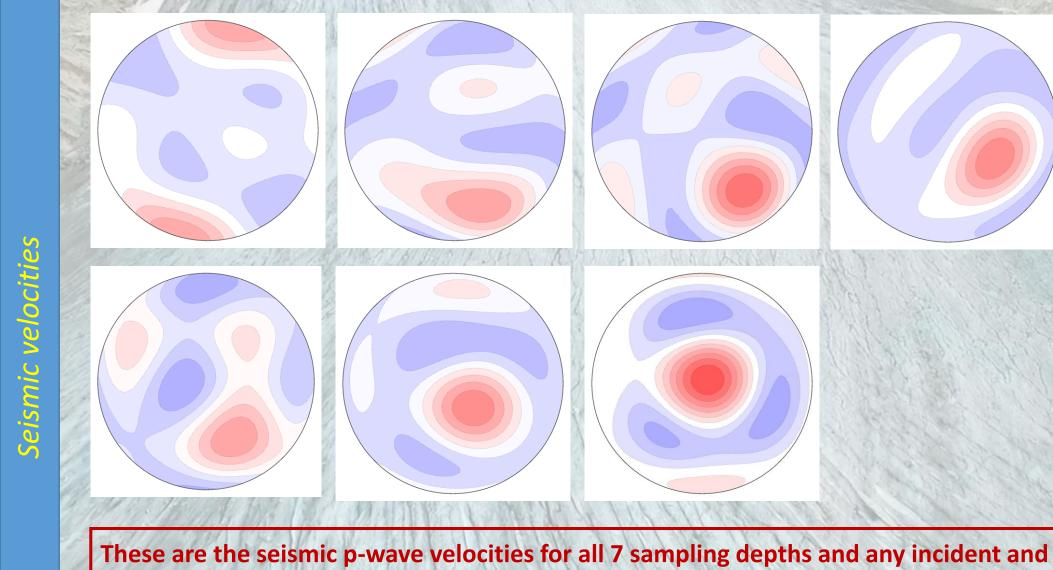
These are the seismic p-wave velocities for all 7 sampling depths and any incident and azimuth angle of a seismic wave. The maximum anisotropy is found for 79 m with 2.3%. The centre of the diamond-shape cluster represents the direction of maximum velocity, the minimum velocity is found around this maximum with an offset of about 45-50°.
