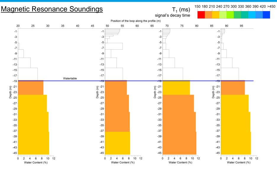
⇒ MRS water content shows significant water content variation above the water table. ⇒ Uniform water content and  $T_1$  under the water table confirm the global tabularity of the limestone massif.
