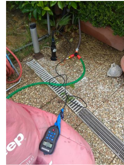
Physical-Chemical parameters measurements in low flow cell
