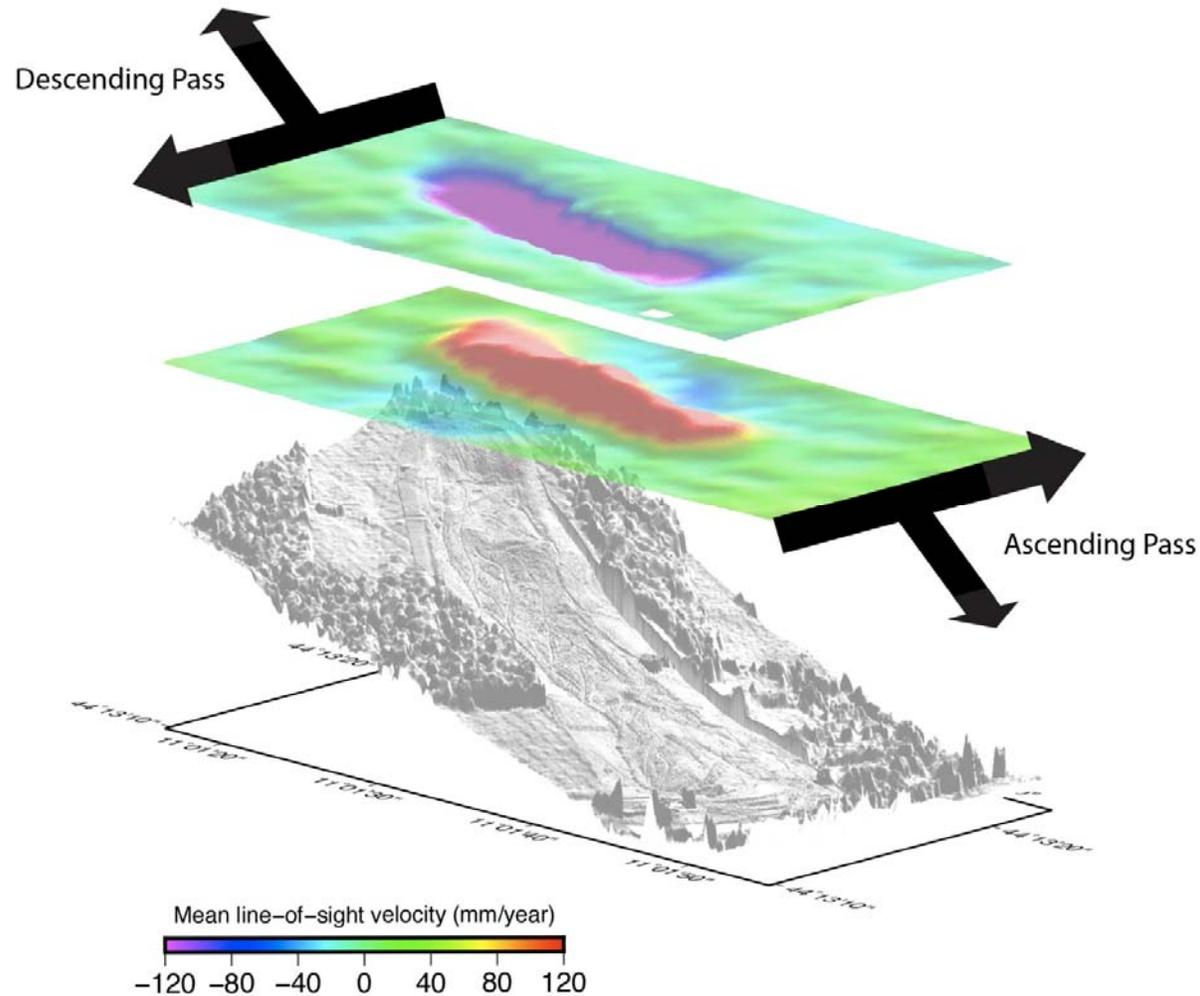
Standard InSAR can be used to maximize the amount of useful displacement information that can be extracted from SAR images.
