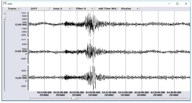
Recorded seismic noise at the station (data available) is shown here for the 3 channels HHZ HHN and HHE:
