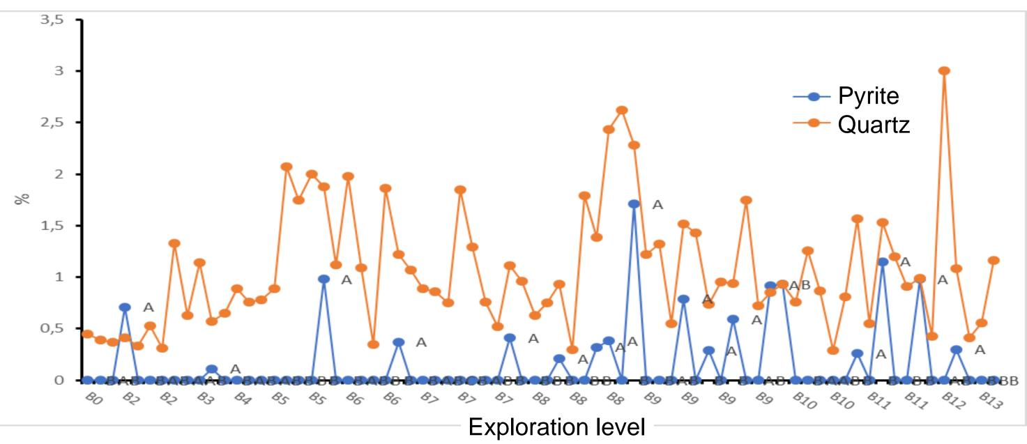
Figure 4: Pyrite and quartz abundance in function of the stratigraphy of the quarry, from B0 (more superficial) to B13 (deeper). A corresponds to darker fractions of the stone.
