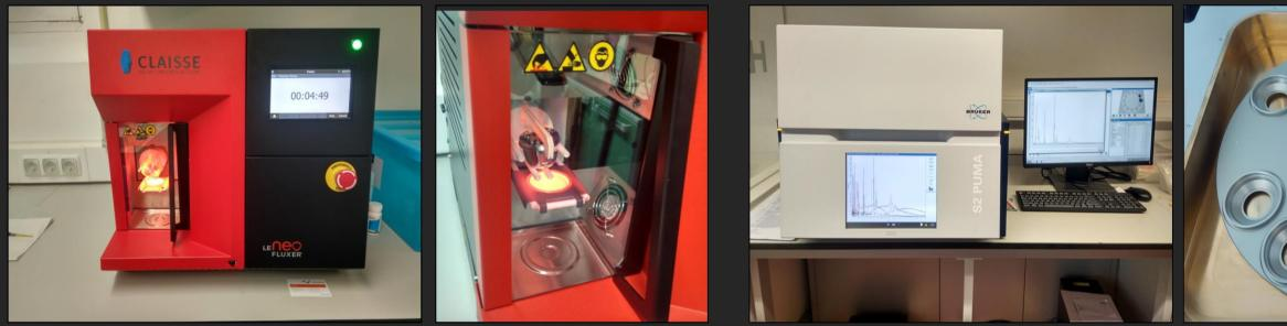
Glass beads preparation, using 12g flux + 1,2g sample
