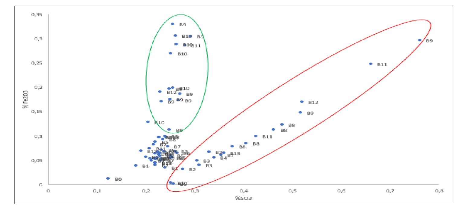
Figure 3:  $Fe_2O_3$  vs  $SO_3$  contents, originating clusters accordingly with the colour of the stone fraction. Lighter fraction – green cluster; Darker fraction – red cluster.
