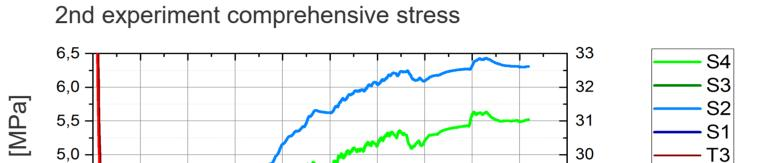
measured the development of temperature, comprehensive stress and expansion within the test construction for approximately one year. During the binding reaction the temperature increased by 55 K in the center.
