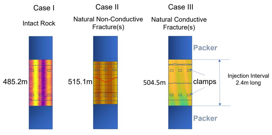
Fracture induced at higher pressure.
