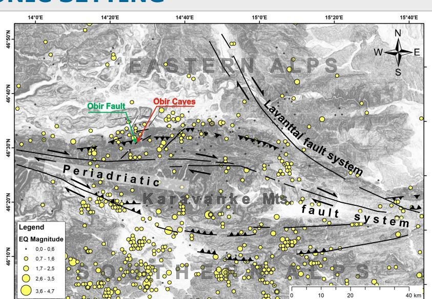
Above: Tectonic setting of the Eastern and Southern Alps transition with the Periadriatic fault system, modified after Baron (et al., 2019a). Yellow dots show earthquake epicentres between 2013 and 2016.
