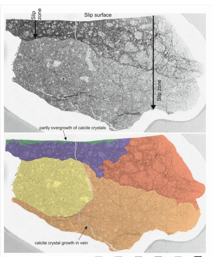
Various cataclastic stages are preserved in the thin section of sample OB8: Besides the undeformed host rock four different stages (I-IV) of cataclastic deformation can be distinguished: (0) undeformed host rock (yellow)
