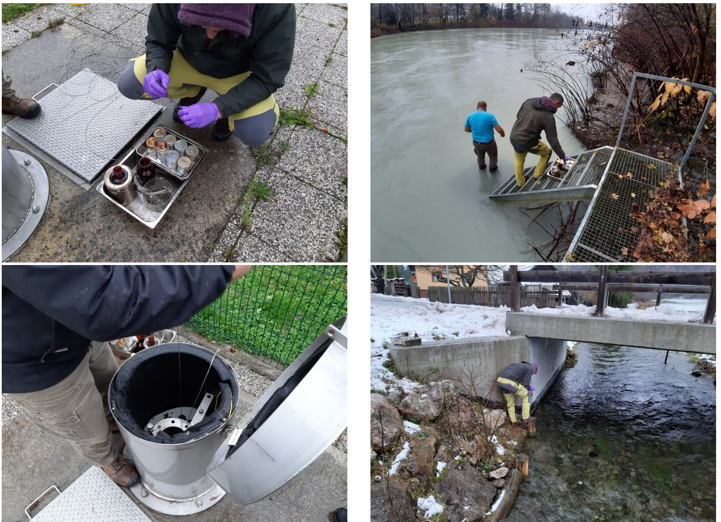
Figure 8, 9, 10, 11: Instalation of passive samplers on surface and groundwater
