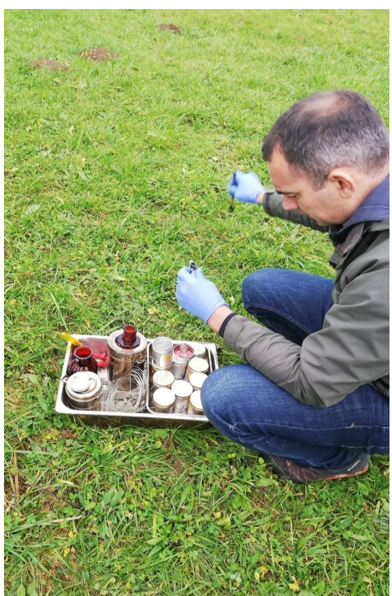
Figure 6: Determination of the presence of compounds that catch on active carbon before installation
