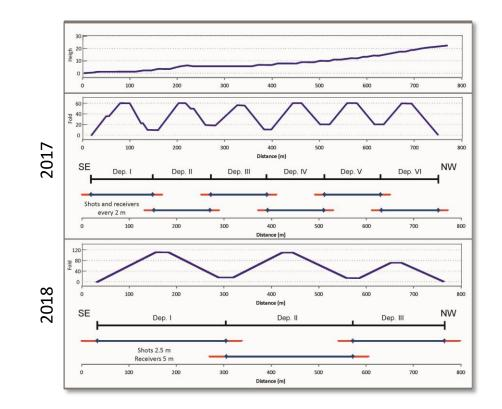
Schematic acquisition geometry Walking deployments with extra offset shots
