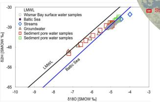
Figure 3 –  $\delta^{18}$ O and  $\delta^{2}$ H of water. Surface water samples of Wismar Bay (circles); sediment pore water samples (squares); Groundwater at the shore line (triangles); Streams discharging into Wismar Bay (diamond); Baltic Sea Line (blue line), Local Meteoric Water Line established to Warnemuende (black line).
