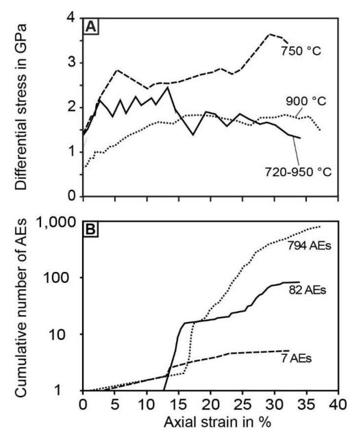
The stress-strain evolution (A) as well as the cumulative number of AEs versus axial strain (B) are shown for the tree experiments that were all performed at 2.5 GPa confining pressure and a strain rate of  $5 \times 10^{-5}$  s<sup>-1</sup> but at different temperatures.
