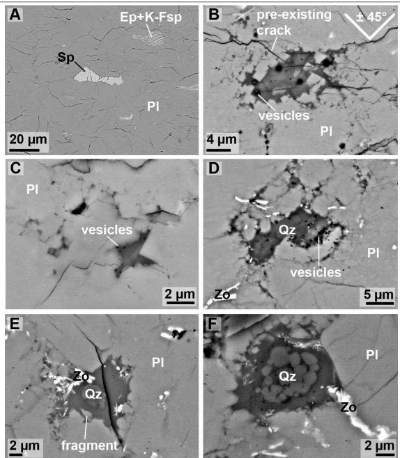
Backscattered-electron images of the recovered deformation samples. The direction of maximum compression ( $\sigma_1$ ) is oriented normal to the long edges of the images.
